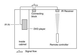
The miniplug cable from the connecting block should be connected to the DVD player's IR IN jack, as shown below.
